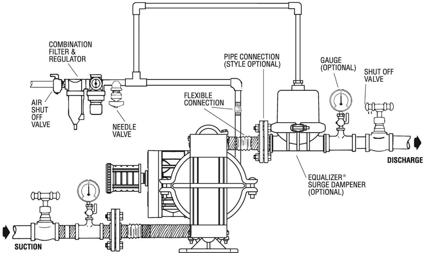
**NOTE:** In the event of a power failure, the shut-off valve should be closed, if the restarting of the pump is not desirable once power is regained.
